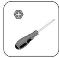
Phillips screwdriver (M4, M6, M8)
